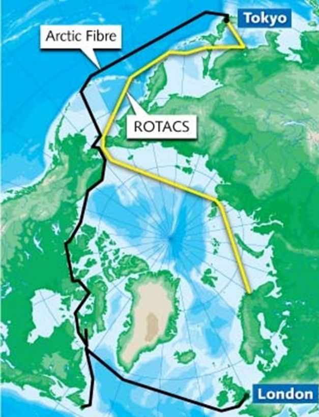
"Polar Express"- a project that has been launched to build an underwater Transarctic fiber-optic cor line (FOCL) connecting Europe and Asia through the Arctic zone of Russia, with exit points along the Northern Sea Route (NSR) and the possibility to include it in the existing FOCL with routes to Europe, Asia and America
