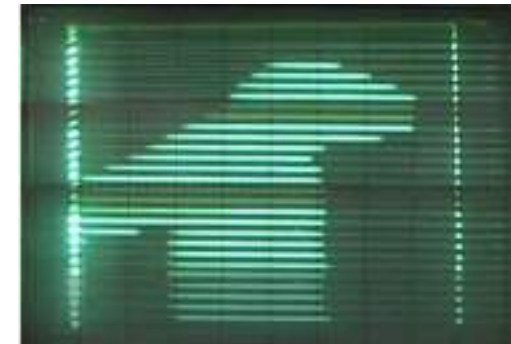
40 scanning lines and a television picture rate of 14 per second
